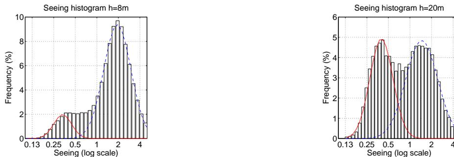
**Fig. 1. Left:** Seeing histogram at an elevation of  $h = 8m$  for the period April to September. **Right:** Idem for  $h = 20m$  from available data in 2005 and 2012. Red (solid) and blue (dashed) lines are Gaussian fit of the two bumps. They give the fraction of time spent by the DIMM inside (blue line) or outside (red line) the SL. At  $h = 20m$  the DIMM is in the free atmosphere 45% of the time (12% at  $h = 8m$ ).
